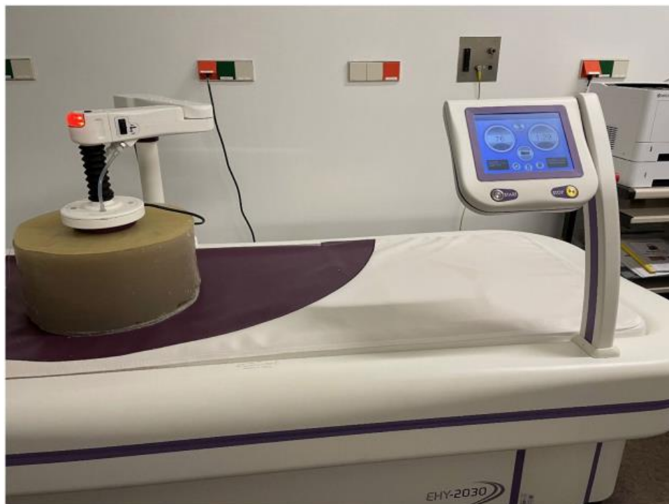
Figure 3. Assembled inhomogeneous phantom during a heating procedure with the EHY-2030. The phantom has 4 parts. A circular agar cylinder (diameter 45 cm, height 20 cm) is built from
