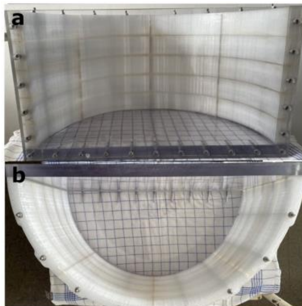
Figure 1. (a) View from the planar side onto the casting mold and (b) view from above onto the casting mold.
