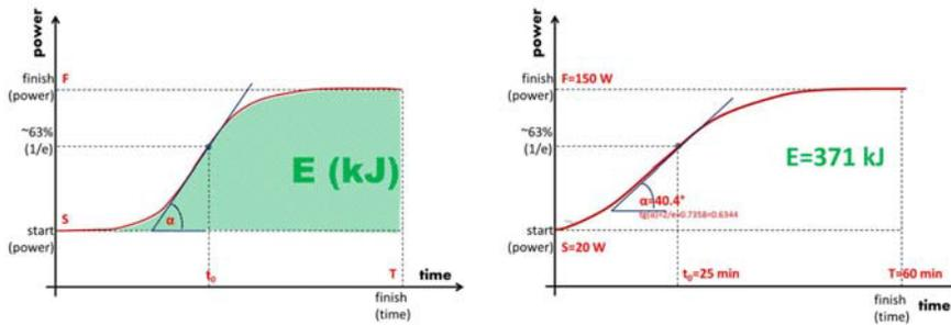
**Figure 2.** The provided energy is represented by the area under the curve (integral of the forwarded power, (a)), and the slope at the inflexion point is proportional with the exponent “a”, shown in numerical example (b)
